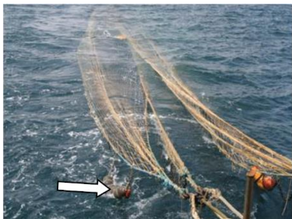
Figure 25: Set-up of DDD-03H on pelagic trawl net; excerpt from De Carlo et al., 2011.
