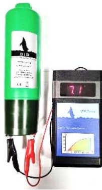
Figure 27: Voltage reading using the STM Volttester. As evidenced in the diagram, the internal batteries must be recharged when the voltage reaches 6V, because below this value the performance of the device is strongly reduced.
