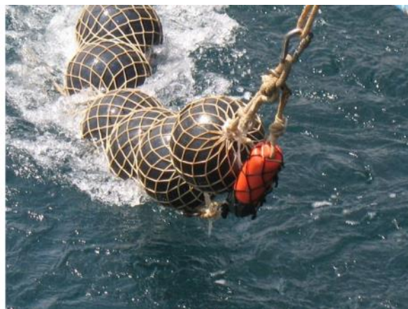
Figure 25: Set-up of DDD-03H on pelagic trawl net; excerpt from De Carlo et al., 2011.
