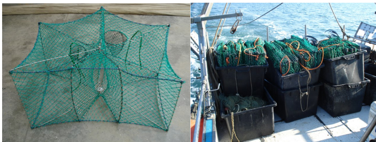
Figure 1. On the left, a photograph of one Trapula pot (three-chambers design), which was tested during the TartaLife project (LIFE12NAT/IT/000937). On the right, a photograph of Trapula pots stored on board a fishing vessel.
